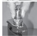
Insert the holder into the press so that the lock groove will line up when secured. Adjust your die in or out for proper operation.
