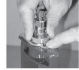
Remove the die by depressing the lock button and rotate the die 1/6 of a turn lift out and change to your next die
