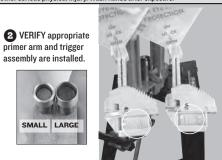
3 MAKE sure trough fingers are between and completely engaged with tray latch lugs (highlighted)
