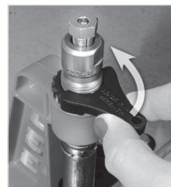
Remove by rotating die 1/6 of a turn counterclockwise; lift out.
